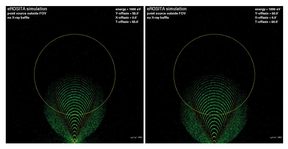
no baffle, no pile-up: bright source off-axis: 55 arcmin (left), 60 arcmin (right)
