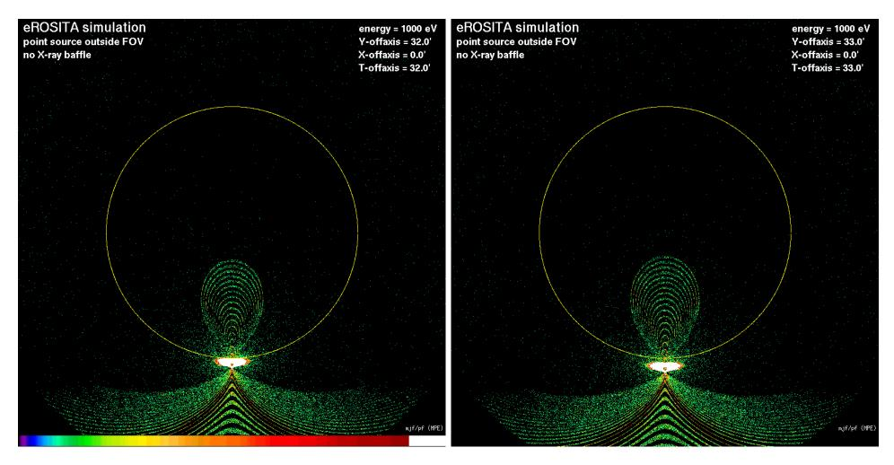
no baffle, no pile-up: bright source off-axis: 32 arcmin (left), 33 arcmin (right)
