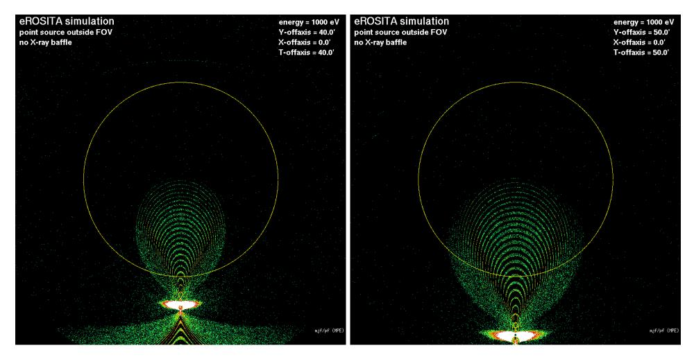
no baffle, no pile-up: bright source off-axis: 40 arcmin (left), 50 arcmin (right)
