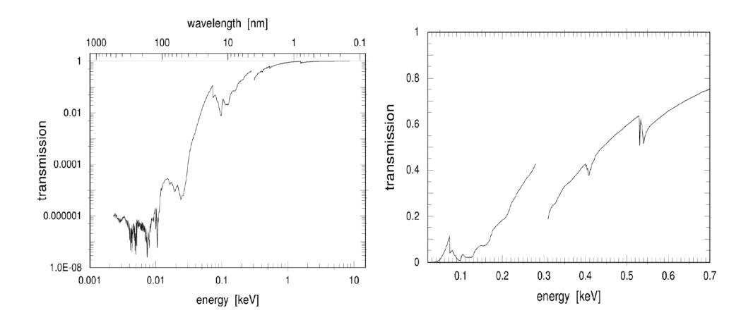
BESSY measurements: degraded performance suspected around C-K edge  $\rightarrow$  no data delivered, gap
