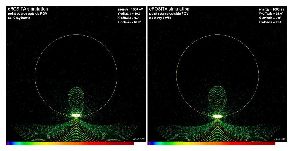
no baffle, no pile-up: bright source off-axis: 30 arcmin (left), 31 arcmin (right)
