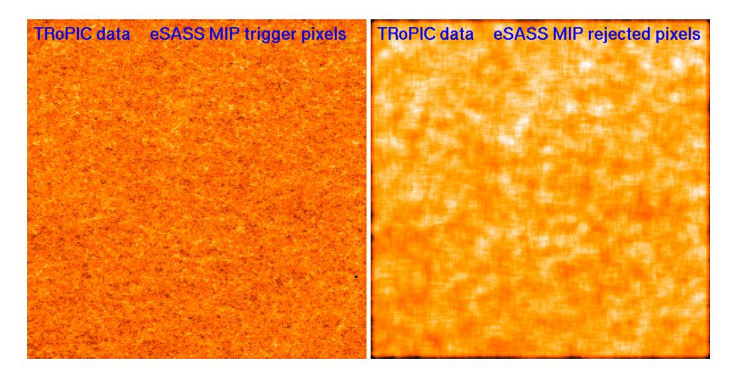
pixels above trigger threshold  $\rightarrow$  pixels rejected by 2D algorithm here: 3 pixels width in each X and Y semi-axis
