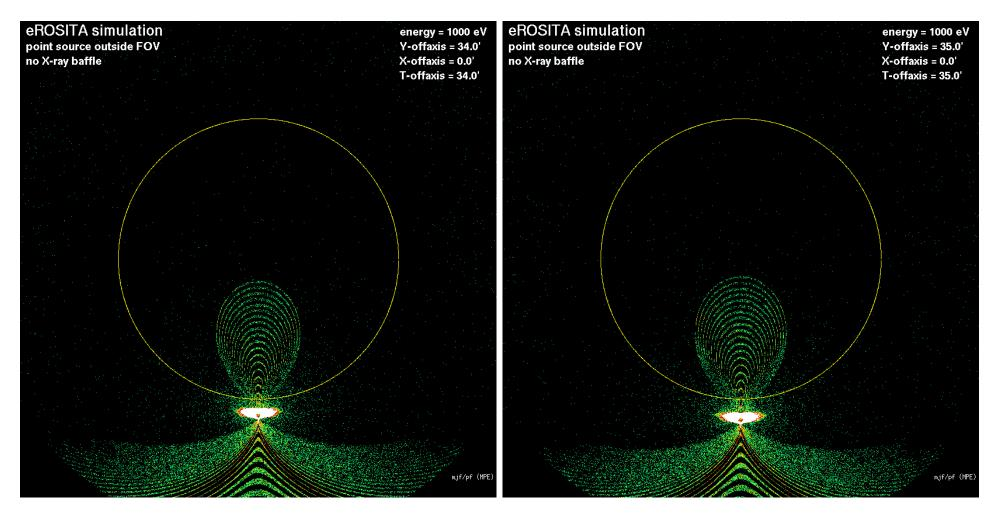
no baffle, no pile-up: bright source off-axis: 34 arcmin (left), 35 arcmin (right)
