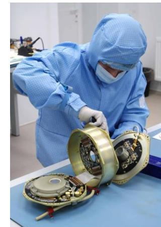
Model mirror system+mylar, effective area on-axis, D=28.56 mm
