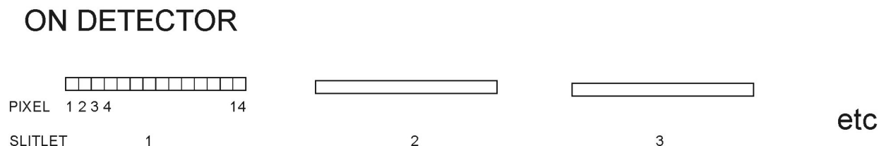
Figure 4 Numbering of pixels and slitlets as they are referenced to in Figure 5
