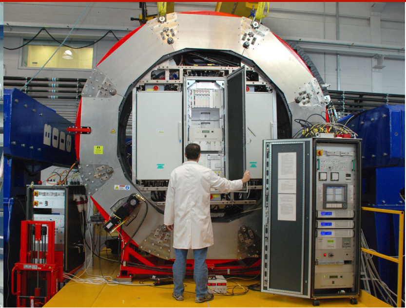
The back: cable derotator & electronic cabinets
