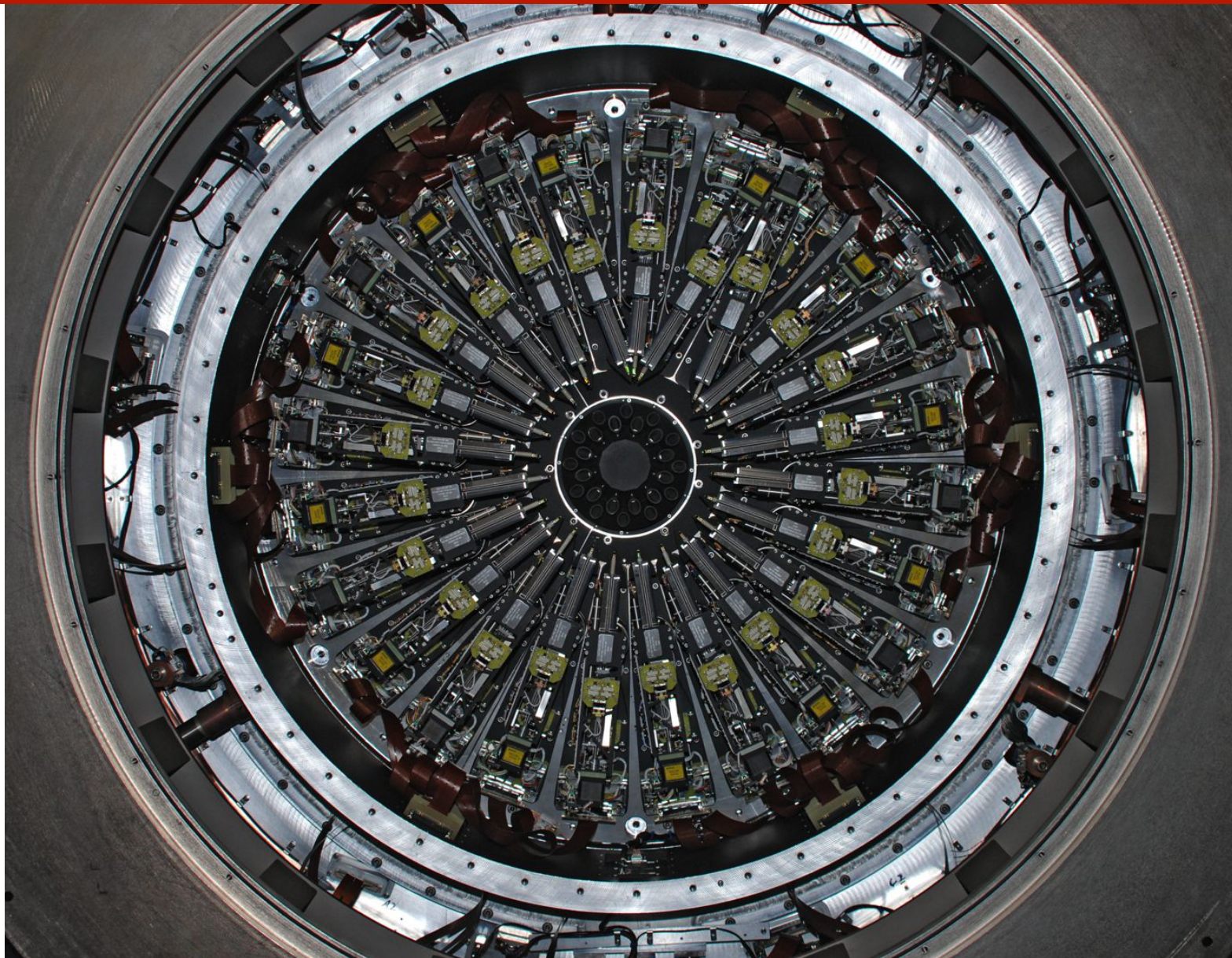
Inside the cryostat: the 24 robotic arms
